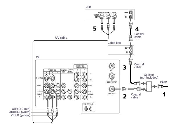
To switch between channels from cable box and channels from CATV
